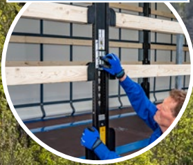
Centre posts can be adjusted with pins
