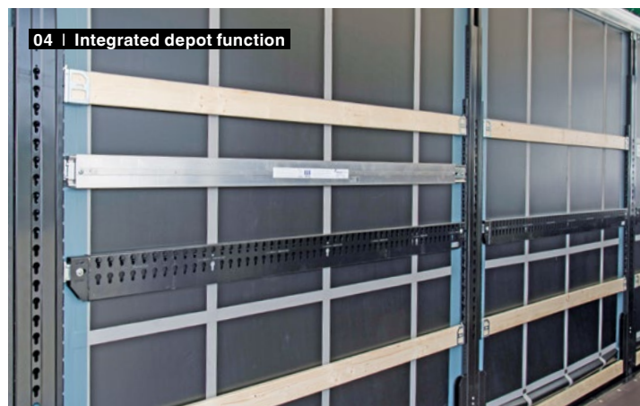
04 | Flexible handling of the lath sockets
