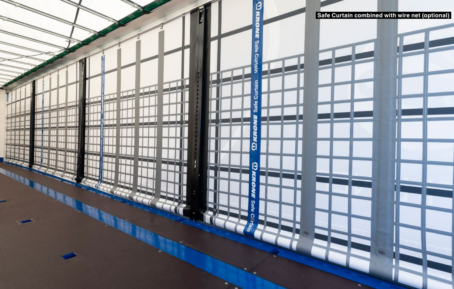
Patented connection of the Spring steel stripes (Safe Curtain)
