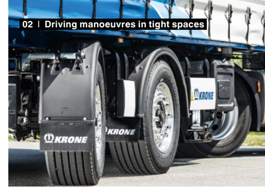
02 | Low-maintenance forced steering
