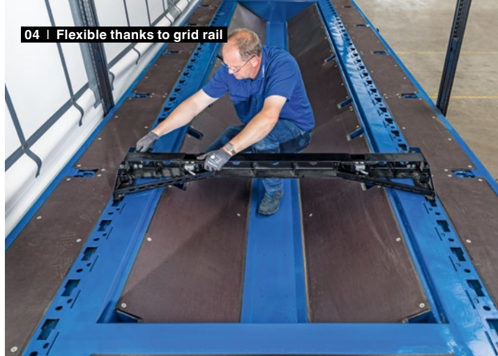
04 | Securing to the rear with crossbeam
