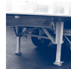
Figure 2.3.1.a. – "Aluminium type" landing leg
