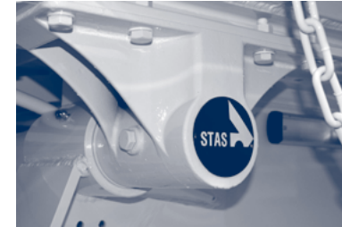
Figure 3.a. – Bolts for tipping shaft locking
