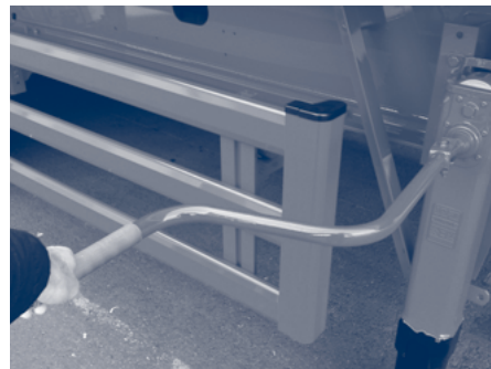
Figure 2.2.1.c. – Landing leg handle "steel type"
