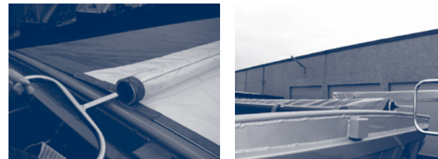
Figure 7.3.2.b. - Operating of Dawnbarn from catwalk
