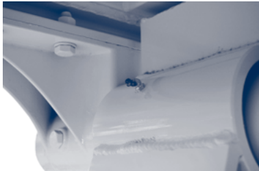
Figure 6.c. - Lubricate tipper turning points
