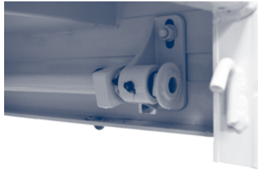
Figure 6.b. - Lubricate the clamping hoods of the top hinged door and universal door
