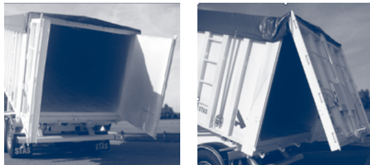
Figure 6.3.1.a. – Universal door as barn door (left) and as top hinged door (right)
