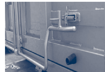
Figure 6.1.2.a. – Closing safety system
