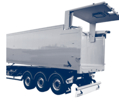
Figure 6.5.1.a. – Tipper with hydraulic top hinged door
