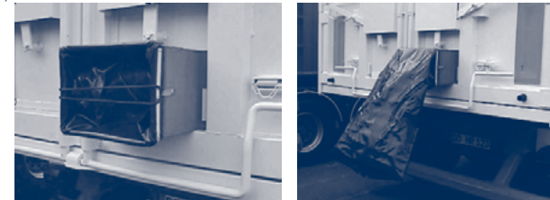
Figure 8.2.1.b. – Door with grain hatch with dust sleeve
