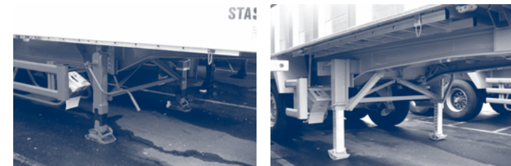
Figure 2.1.a. – “Steel type” (left) and (right) “aluminium type with two landing legs”
