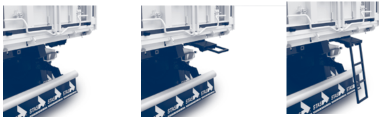
Figure 10.2.a. – Ladder (optional) for access to loading area
