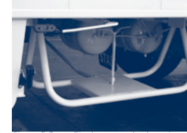
Figure 5.2.a. – Single spare wheel carrier
