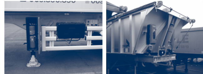
Figure 8.7.a. – Location of fire extinguisher on the tipper
