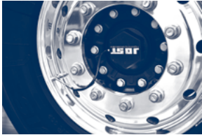
Figure 5.4.b. Air hose from hub to valve in a TPRS system.
