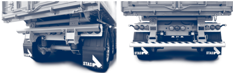
Figure 8.4.1.b. – Automatic hinged rear under-run bar
