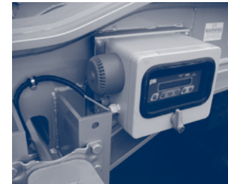
Figure 8.5.1.a. – Weighing equipment measuring unit
