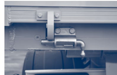
Figure 6.2.2.a. – Safety catch locking hooks top hinged door (unlocked left; locked right)
