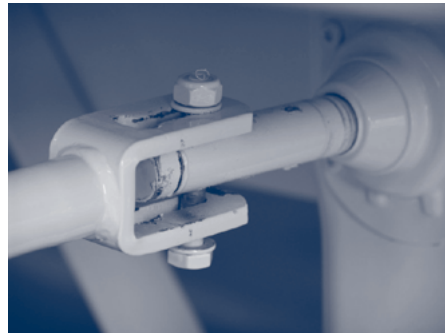
Figure 2.2.1.b. – Landing leg handle "steel type" pulled out
