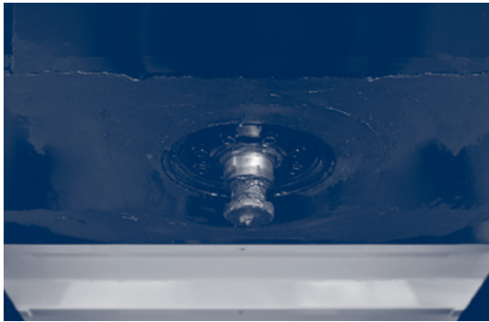
Figure 1.a. – Fifth wheel rubbing plate with kingpin
